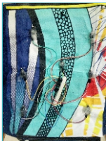
Vibrating sensors connection to base material
